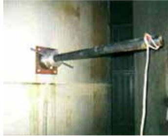
Cardox tube is placed in the tube holder, inserted and then secured in the socket. The tube is then activated.
